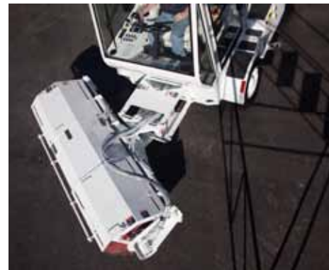
Broom head can pivot 33 degrees to each side.
