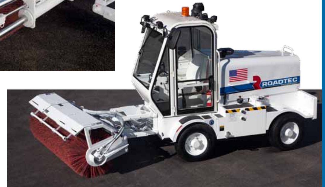
The broom drive motor can be switched to the right or left side to allow right-hand as well as left-hand flush-sweeping.
