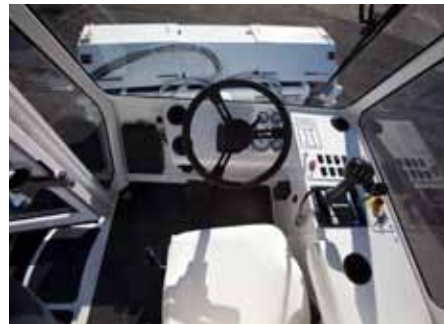
Left-hand side entry, pressurized cab with easy to use controls, filtered climate control, and windshield wiper/washer.
