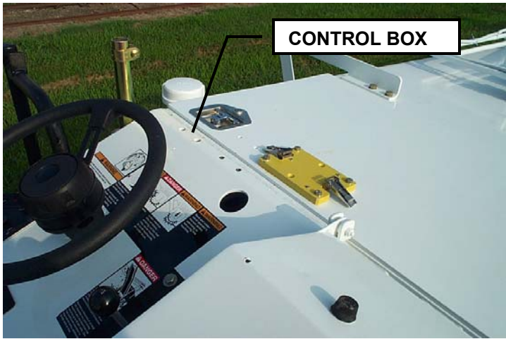
Control Box ( Console Location )
